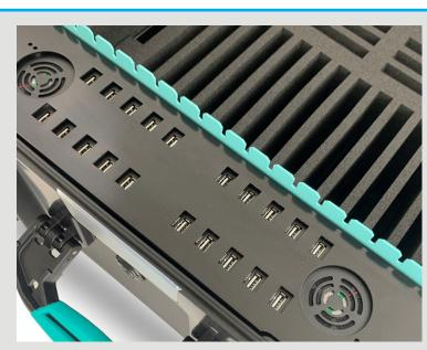
Intelligent charging hub with autom. shut down (no Timer needed) -> works as overheating and overchar ging protection
